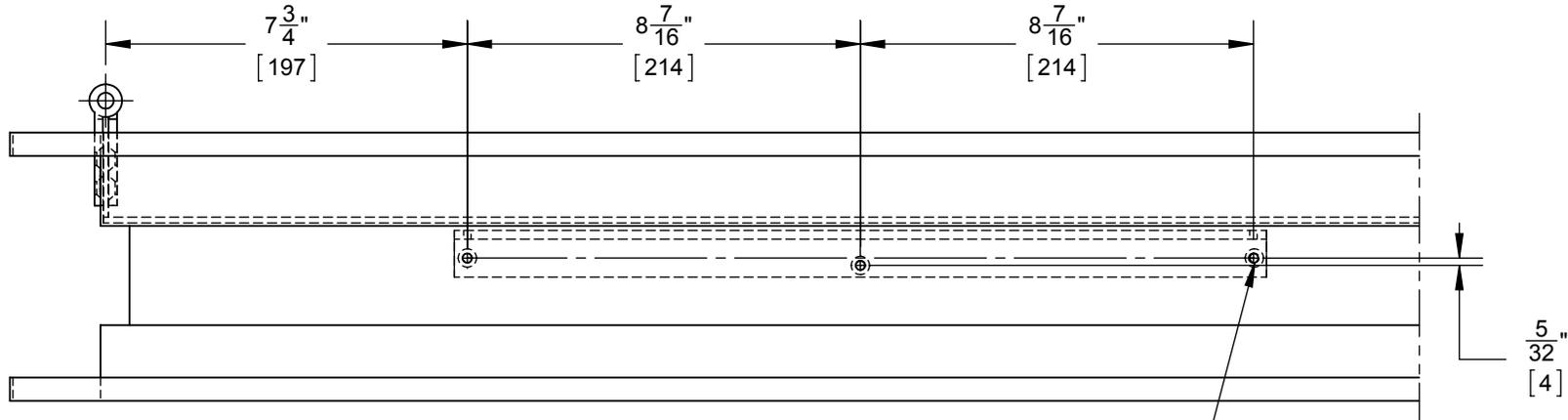
10-32 MACHINE SCREWS, USE No. 21 ( $\phi$ .159") DRILL AND TAP.
