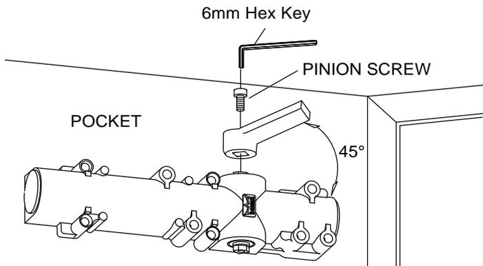
4 Attach arm shoe to door. Adjust connecting arm rod length according to pocket depth chart and tighten screw.
