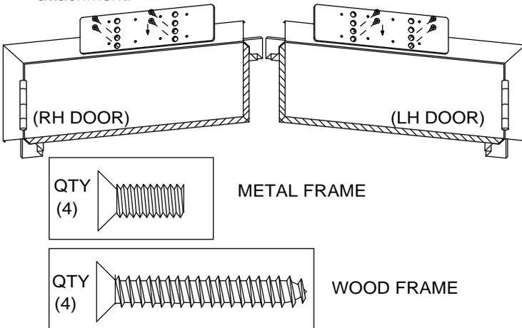
3 Attach closer to frame or plate with spring adjustment facing hinges.
