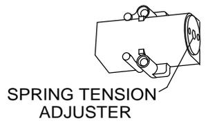
**8916 ONLY BARRIER-FREE OPENINGS -** Take an opening force reading from the pull on the door. If required, adjust the spring tension to meet the barrier-free requirement. Maximum number of turns counter clockwise=8. Maximum number of turns clockwise =14. Depending on opening conditions, a door adjusted to meet barrier-free forces may not have sufficient power to reliably close and latch the door.
