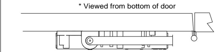
With main arm parallel to door, place main arm onto bottom pinion. Fasten securely with pinion screw.
