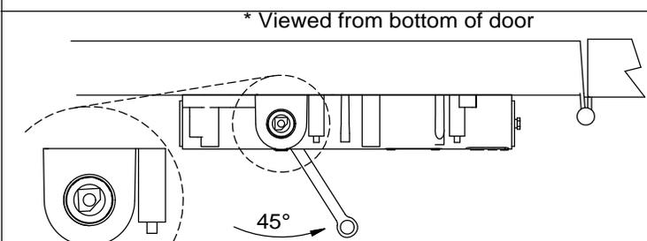
Rotate pinion 45° TOWARD HINGE edge of door.
