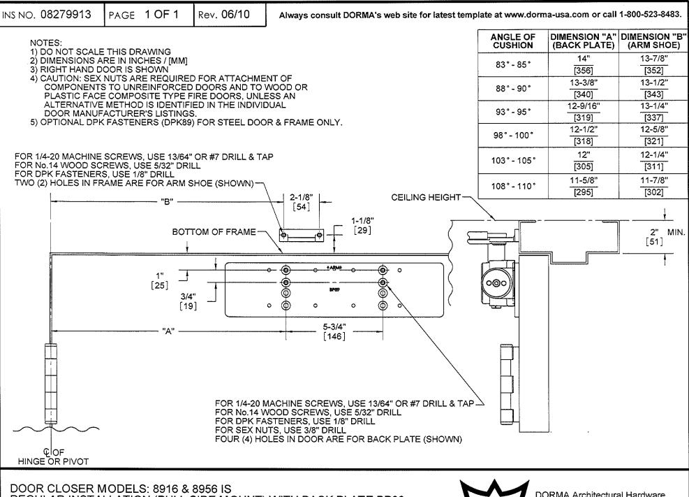
REGULAR INSTALLATION (PULL SIDE MOUNT) WITH BACK PLATE BP89 INTEGRA CUSHION ARM
