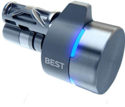
The Switch Tech core is a small-format interchangeable core that can quickly convert a standard door into an electronic access control door. The Switch Tech Core replaces the keyhole mechanism - so you will no longer use a physical key to open the door. Instead, access is granted using the Best Switch app or the Keri Key Switch app on your phone and a Borealis-registered Bluetooth mobile credential.
