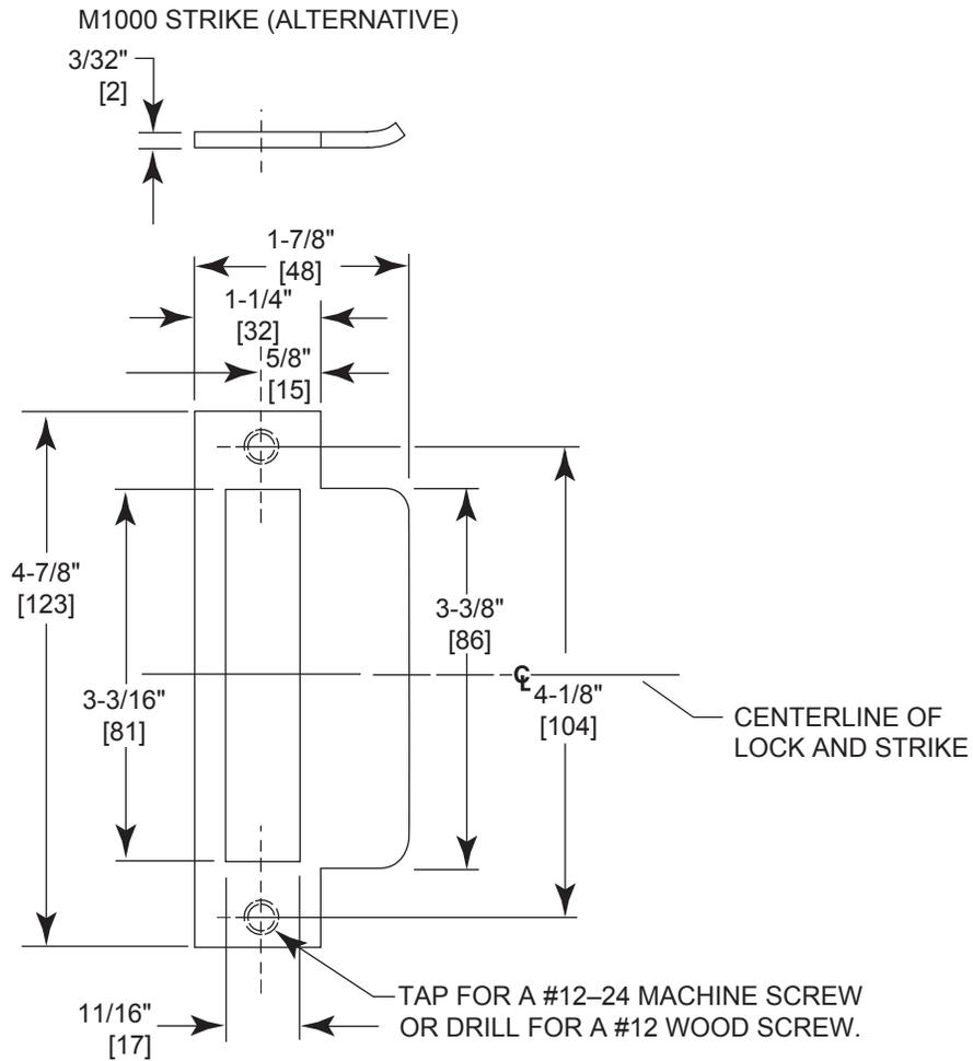
NOT TO SCALE. MEASUREMENTS ARE FOR REFERENCE ONLY. NOT A DRILLING TEMPLATE.
