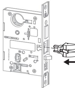
4.2.6 Reinstall latch bolt set screw and tighten securely.
