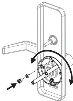
4.4.4 Rotate lever and liner assembly 180° relative to the escutcheon.
