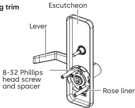
4.4.1 Remove 8-32 Phillips head screw and spacer.
