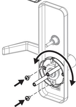
4.4.4 Rotate lever and liner assembly 180° relative to escutcheon.
