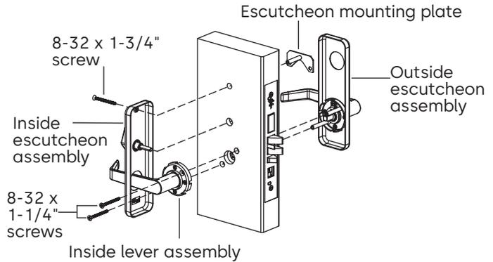
**NOTE: Ensure spindle and thumb turn engage mortise chassis.**
