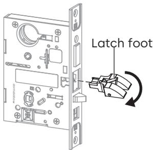
4.2.5 Reinstall latch into lock.
