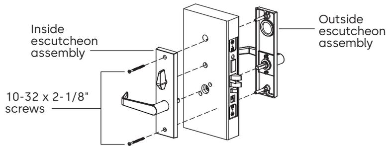
**NOTE: Ensure that spindle and thumb turn engage mortise chassis.**
