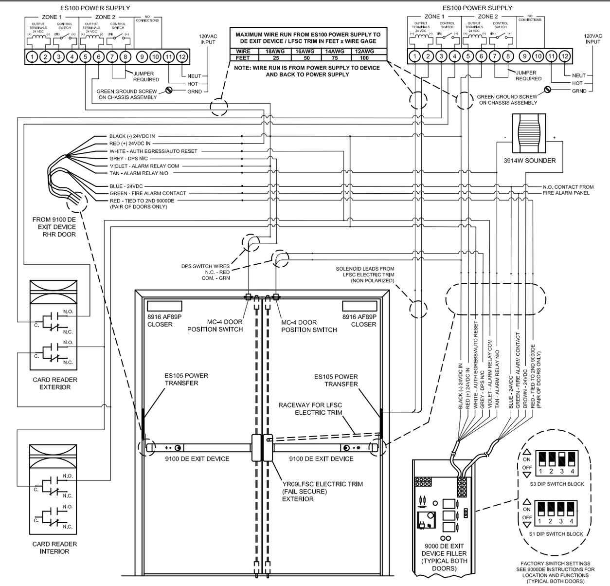
NOTE: This wiring diagram is provided to assist in interfacing DORMA USA products into the system described above. Compatibility and functionality of components not supplied by DORMA are not guaranteed. Component failure resulting from improper wiring is not covered by warranty. Refer to individual device product information sheets and installation instructions for wire gauge sizes and additional information.
