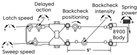
8900 series has a unique footprint. The mounting holes are not at the ends of the body. One pair is close to the spindle.
