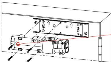
TS93 series always has a track arm, and is attached using a mounting plate that goes on the door first. It has a three part cover.
