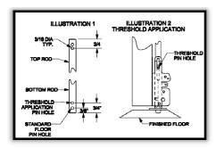
Step 2: Place device into holdback by pushing on touchbar. Clearance between the bottom of the bolt and the surface where strike will be mounted should be ¼". If clearance is not ¼", remove rod pin and thread rod into or out of the rod carriage to achieve ¼" clearance. Install rod pin and spring clip.
