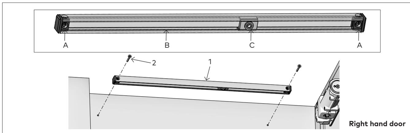
2.3.1 Position the end block inside the track channel (1).
