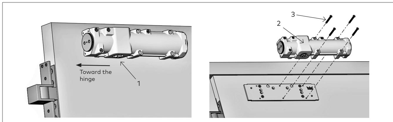
**NOTE:** Orient pinion (1) closest to hinge.
