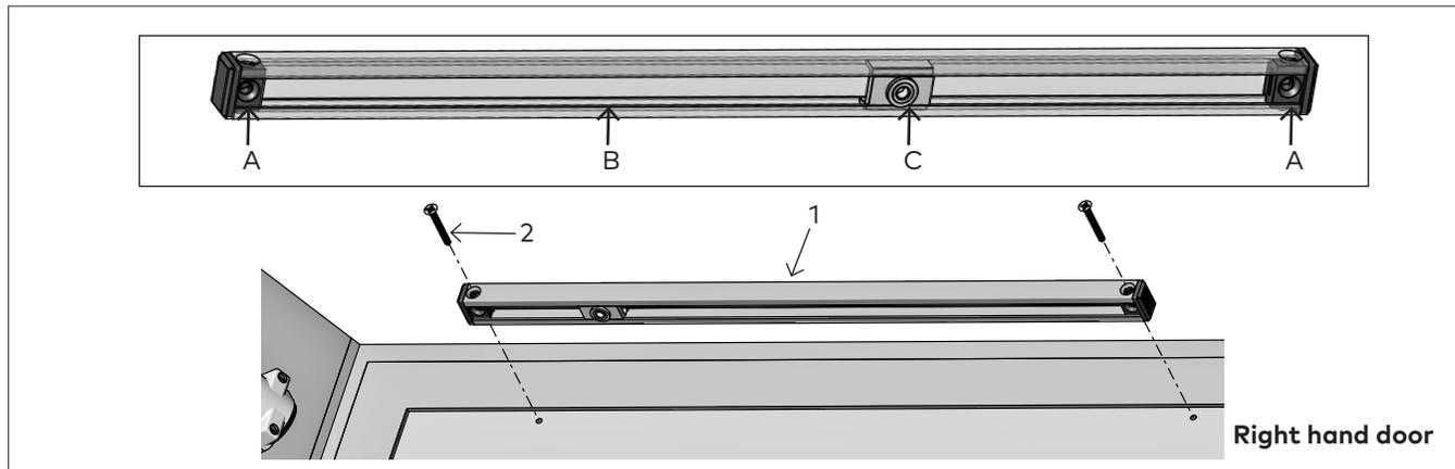
2.3.1 Position the components inside the track channel (1).
