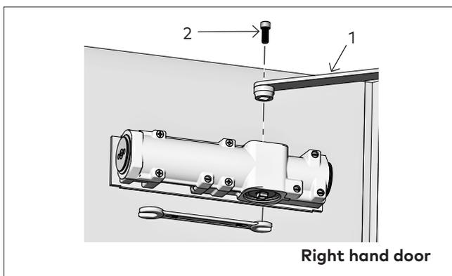
2.5.1 With the door closed and using an adjustable wrench (looking up at the bottom of the closer):
