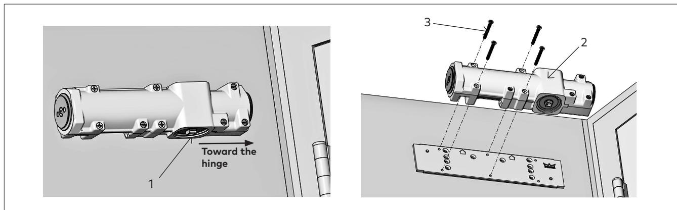
**NOTE:** Orient pinion (1) closest to hinge.
