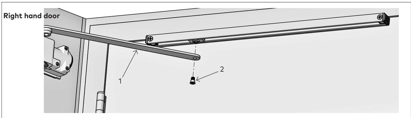
2.4.1 Align the arm (1) with the slide shoe of the track channel.
