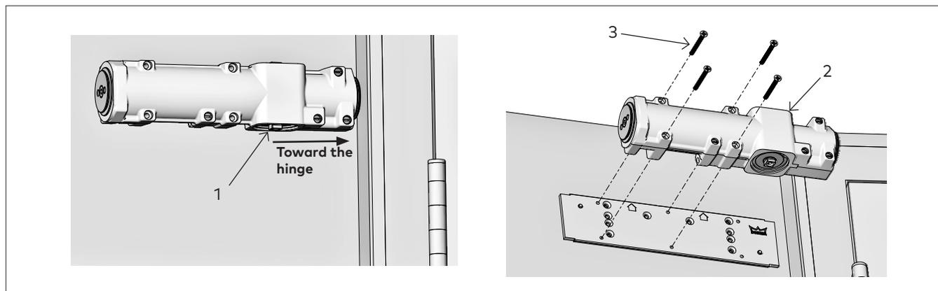
**NOTE:** Orient pinion (1) closest to hinge.
