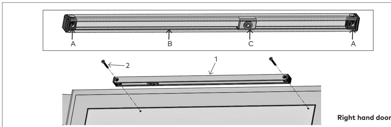
2.3.1 Position the components inside the track channel (1).
