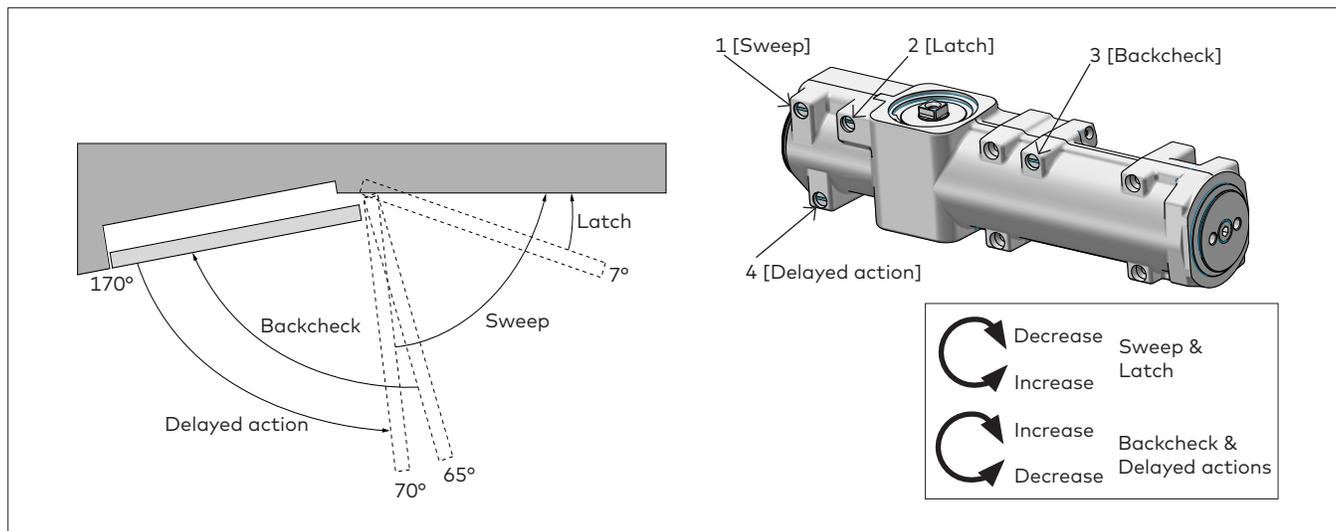
3.1.1 Adjust the **closing sweep speed** (1) for the area from 70° - 0°
