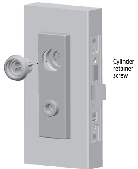
Figure 14b Installing the high-security cylinder
