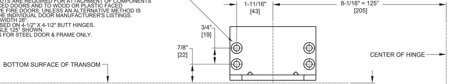
FOR 1/4-20 MACHINE SCREWS, USE 13/64" OR #7 DRILL & TAP
