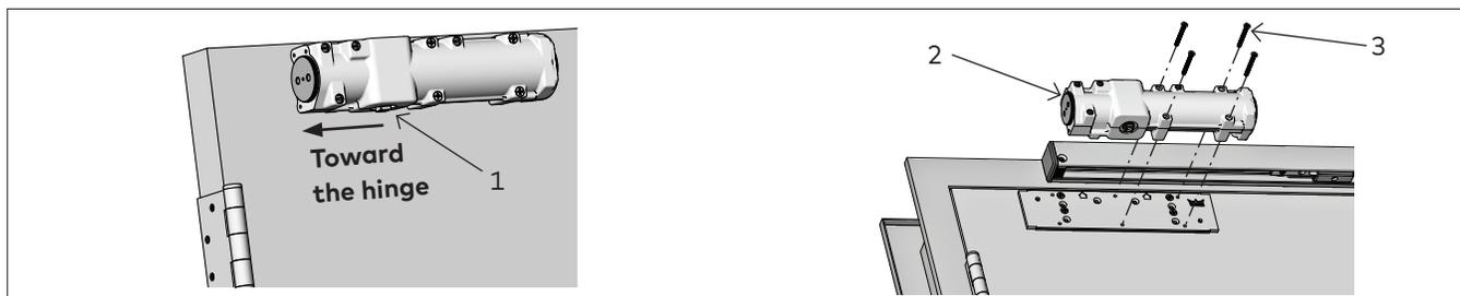
NOTE: Orient pinion (1) closest to hinge.
