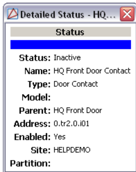
Figure 16.80. Door Contact Detailed Status
