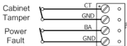
Figure 20.81. Hardware OP16 Inputs
