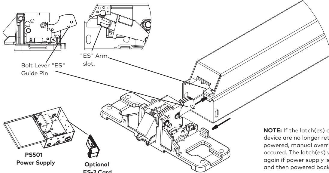
**NOTE:** If the latch(es) on the ES9000 device are no longer retracted while powered, manual override may have occurred. The latch(es) will only retract again if power supply is disconnected and then powered back up.
