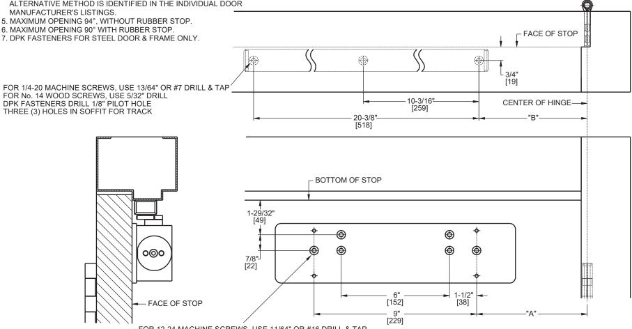
FOR 12-24 MACHINE SCREWS, USE 11/64" OR #16 DRILL & TAP FOR No. 12 WOOD SCREWS, USE 9/64" DRILL DPK FASTENERS DRILL 1/8" PILOT HOLE FOR SEX NUTS USE 3/8" DRILL
