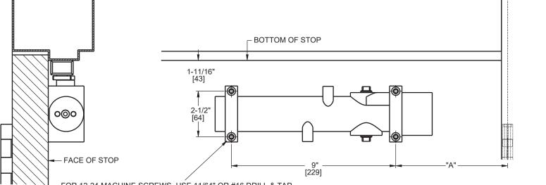
FOR 12-24 MACHINE SCREWS, USE 11/64" OR #16 DRILL & TAP FOR No. 12 WOOD SCREWS, USE 9/64" DRILL DPK FASTENERS DRILL 1/8" PILOT HOLE FOR SEX NUTS USE 3/8" DRILL
