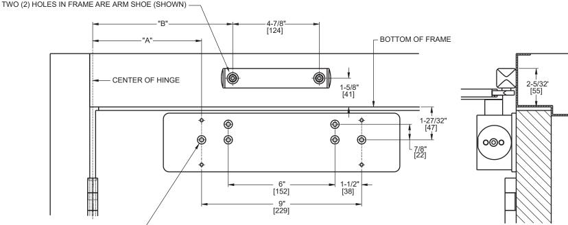
FOR 12-24 MACHINE SCREWS, USE 11/64" OR #16 DRILL & TAP FOR No. 12 WOOD SCREWS, USE 9/64" DRILL FOR DPK FASTENERS, USE 1/8" DRILL FOR SEX NUTS, USE 3/8" DRILL SIX (6) HOLES IN DOOR ARE FOR BACK PLATE (SHOWN)
