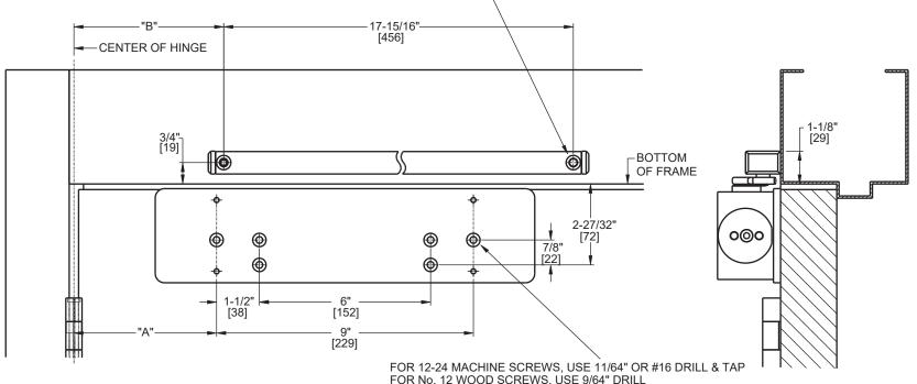
FOR 12-24 MACHINE SCREWS, USE 11/64" OR FOR No. 12 WOOD SCREWS, USE 9/64" DRILL DPK FASTENERS DRILL 1/8" PILOT HOLE FOR SEX NUTS USE 3/8" DRILL SIX (6) HOLES IN DOOR FOR PLATE (SHOWN)
