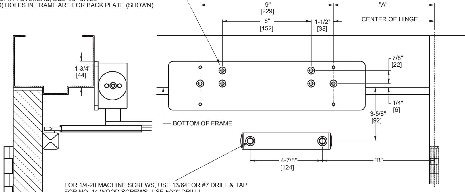
FOR 1/4-20 MACHINE SCREWS, USE 13/64" OR #7 DRILL & TAP
