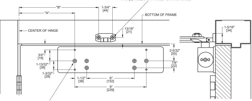
FOR 12-24 MACHINE SCREWS, USE 11/64" OR #16 DRILL & TAP FOR No. 12 WOOD SCREWS, USE 9/64" DRILL DPK FASTENERS DRILL 1/8" PILOT HOLE FOR SEX NUTS USE 3/8" DRILL SIX (6) HOLES IN DOOR FOR PLATE
