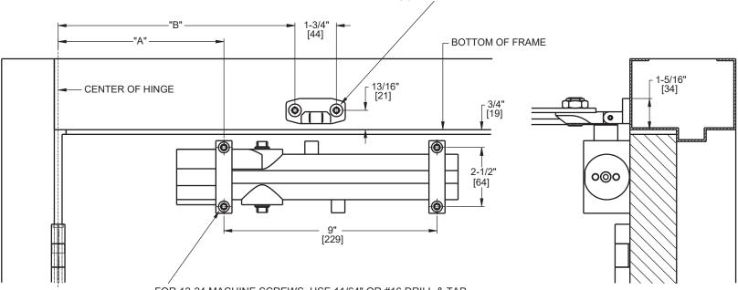
FOR 12-24 MACHINE SCREWS, USE 11/64" OR #16 DRILL & TAP FOR No. 12 WOOD SCREWS, USE 9/64" DRILL DPK FASTENERS DRILL 1/8" PILOT HOLE FOR SEX NUTS USE 3/8" DRILL FOUR (4) HOLES IN DOOR FOR CLOSER
