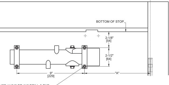
FOR 12-24 MACHINE SCREWS, USE 11/64" OR #16 DRILL & TAP FOR No. 12 WOOD SCREWS, USE 9/64" DRILLL
