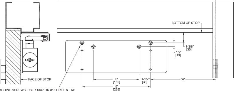
FOR 12-24 MACHINE SCREWS, USE 11/64" OR #16 DRILL & TAP FOR No. 12 WOOD SCREWS, USE 9/64" DRILL FOR DPK FASTENERS, DRILL 1/8" PILOT HOLE FOR SEX NUTS. USE 3/8" DRILL
