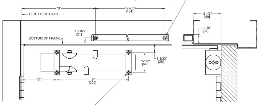
FOR 12-24 MACHINE SCREWS, USE 11/64" OR #16 DRILL AND TAP FOR No. 12 WOOD SCREWS, USE 9/64" DRILL FOR DPK FASTENERS, USE 1/8" DRILL FOR SEX NUTS, USE 3/8" DRILL FOUR (4) HOLES IN DOOR ARE FOR CLOSER (SHOWN)
