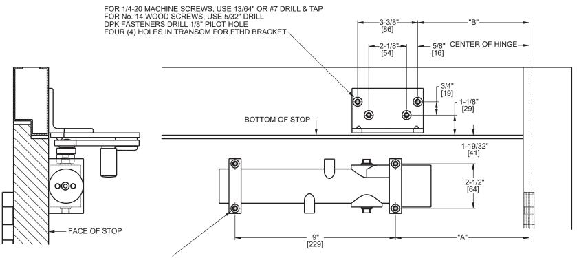
FOR 12-24 MACHINE SCREWS, USE 11/64" OR #16 DRILL & TAP FOR No. 12 WOOD SCREWS, USE 9/64" DRILL DPK FASTENERS DRILL 1/8" PILOT HOLE FOR SEX NUTS USE 3/8" DRILL FOUR (4) HOLES IN DOOR FOR CLOSER
