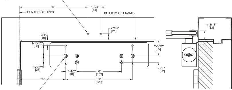
FOR 12-24 MACHINE SCREWS, USE 11/64" OR #16 DRILL & TAP
