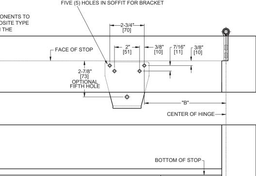
FOR 1/4-20 MACHINE SCREWS. USE 13/64" OR #7 DRILL & TAP
