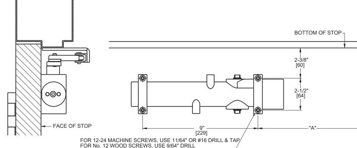
FOR DPK FASTENERS, DRILL 1/8" PILOT HOLE
