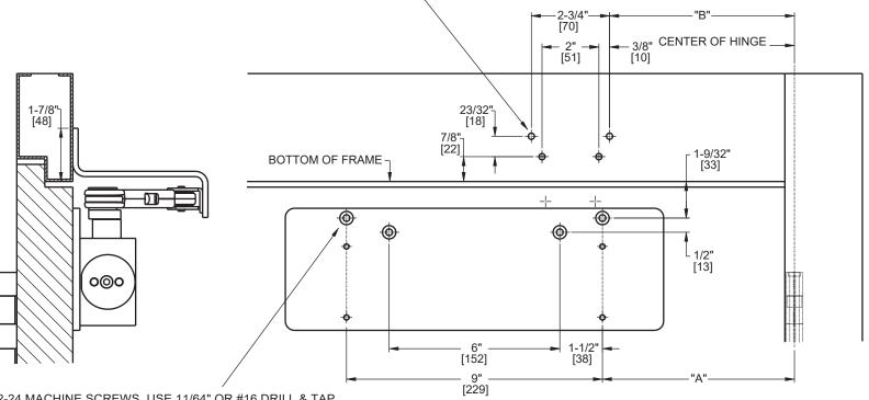
FOR 12-24 MACHINE SCREWS, USE 11/64" OR #16 DRILL & TAP FOR No. 12 WOOD SCREWS, USE 9/64" DRILL DPK FASTENERS DRILL 1/8" PILOT HOLE FOR SEX NUTS USE 3/8" DRILL FOUR (4) HOLES IN DOOR FOR PLATE
