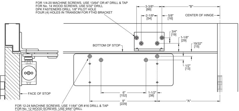
DPK FASTENERS DRILL 1/8" PILOT HOLE FOR SEX NUTS USE 3/8" DRILL FOUR (4) HOLES IN DOOR FOR PLATE
