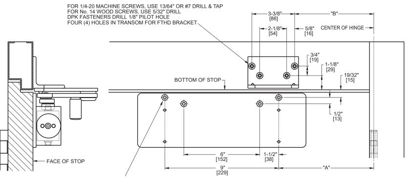
FOR 12-24 MACHINE SCREWS, USE 11/64" OR #16 DRILL & TAP FOR No. 12 WOOD SCREWS, USE 9/64" DRILL
