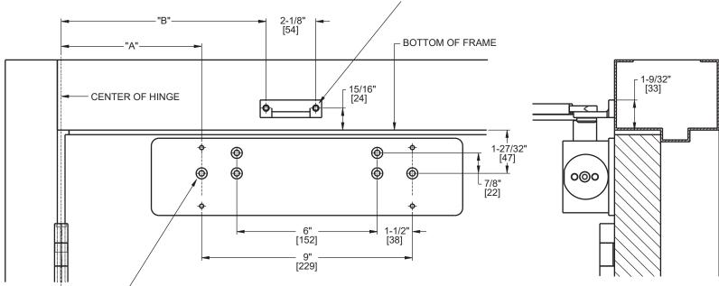
FOR 12-24 MACHINE SCREWS, USE 11/64" OR #16 DRILL & TAP
