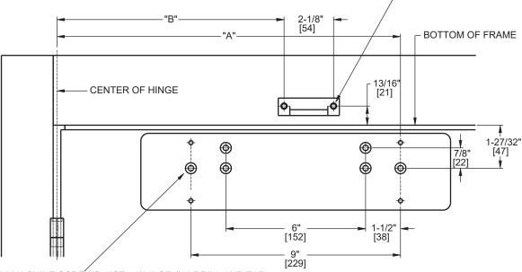
FOR 12-24 MACHINE SCREWS, USE 11/64" OR #16 DRILL AND TAP FOR No. 12 WOOD SCREWS, USE 9/64" DRILL FOR DPK FASTENERS, USE 1/8" DRILL FOR SEX NUTS, USE 3/8" DRILL SIX (6) HOLES IN DOOR ARE FOR PLATE (SHOWN)
