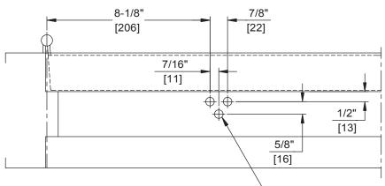
FOR 1/4-20 MACHINE SCREWS USE 7/32" DRILL & TAP → FOR No.14 WOOD SCREWS USE 5/32" DRILL DPK FASTENERS DRILL 1/8" PILOT HOLE THREE (3) HOLES IN SOFFIT FOR BRACKET
