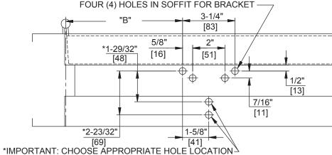
FOR SPACER BLOCK, IN ACCORDANCE WITH FRAME WIDTH.
