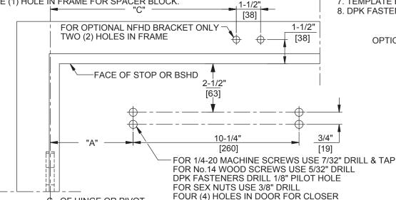
**ANGLE** DIM. "C" DIM. "B" DIM. "A" OF (NFHD) SOFFIT **OPENING CLOSER BRACKET PLATE** HOLD OPEN **OPTIONAL** 6-5/8" 10-1/8" 11" TO 100° [279] H.O. 90° [168] [257] 6-1/2" 3" 7-3/8" TO 180° [76] H.O. 125° [165] [187]
